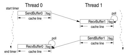
Figure 2.1: Ping-Pong test between two threads using four buffers
