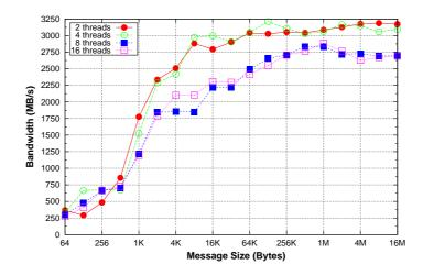
Figure A.2: Bandwidth on Sandy Bridge using multi-line ping-pongs among pairs of threads grouped
