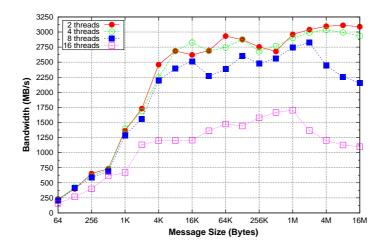
Figure A.4: Bandwidth on Sandy Bridge using multi-line ping-pongs among pairs stressing the QPI link between both processors
