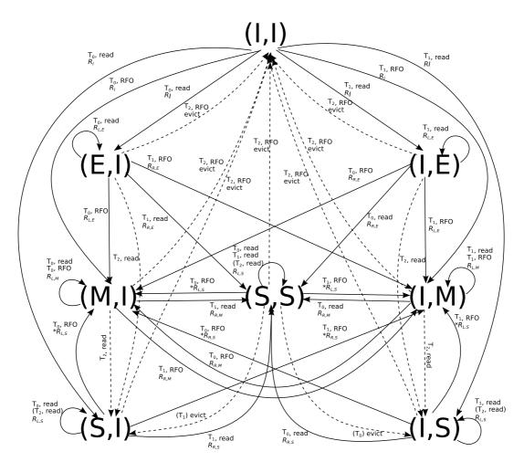
Figure 1.3: Graph of the MESI transitions of a line within two cores
