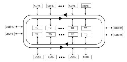
Figure 1.1: Architecture of the Intel Xeon Phi coprocessor
