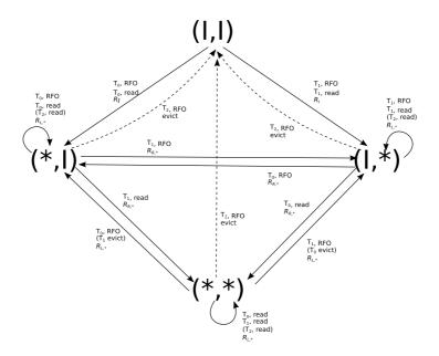
Figure 1.4: Graph of the simplified MESI transitions of a line within two cores
