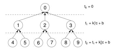
Figure 4.2: Tree for an 10-threads broadcast assuming  $d = 2, k_1 = 3, k_2 = 2$ .
