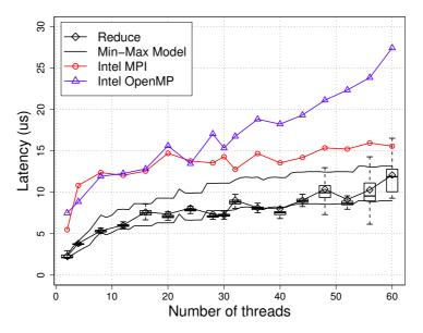
Figure 4.8: Small Reduction performance compared to the model and the Intel OpenMP and MPI implementations
