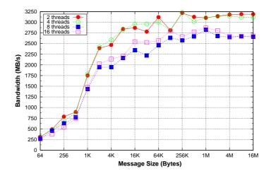
Figure A.3: Bandwidth on Sandy Bridge using multi-line ping-pongs among pairs stressing one link inside each processor.
