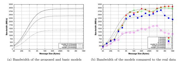
Figure A.8: Bandwidth models for Sandy Bridge when communications are performed across the QPI link
