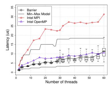
Figure 4.7: Barrier Synchronization results compared to the model and the Intel OpenMP and MPI implementations.
