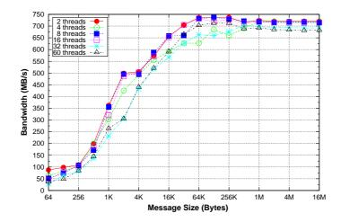
Figure A.10: Bandwidth on Xeon Phi using multi-line ping-pongs among pairs of threads grouped
