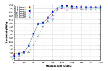
Figure A.11: Bandwidth on Xeon Phi using multi-line ping-pongs among pairs stressing one link
