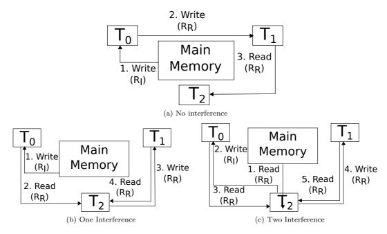
Figure 4.1: Interference in the access to a cache line by two writers  $(T_0 \text{ and } T_1)$  and a reader that is polling the line waiting for writes.
