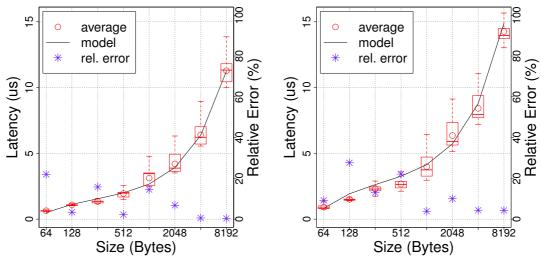
(a) Sender and receiver buffers in Exclusive state. The parameters of the model (in nanoseconds) are  $76.0 \cdot N + 1521.0 - \frac{1096.0}{N}$
