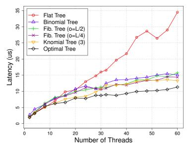
Figure 4.4: Small Broadcast performance comparing our optimal algorithm with widely used broadcast trees.
