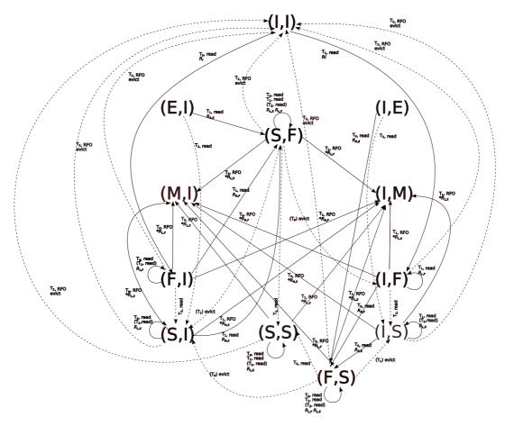
Figure 1.6: Graph of the S and F MESIF protocol transitions of a line within two cores
