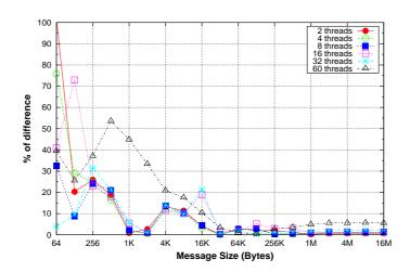
Figure A.13: Percentage of difference between real results and the Xeon Phi bandwidth model.
