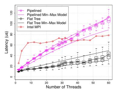
Figure 4.6: Large Broadcast (8 kb) algorithms compared to the model and the Intel MPI implementation.
