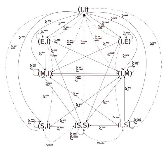
Figure 1.5: Graph of the MESI protocol transitions of a line within two cores
