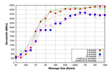
Figure A.5: Bandwidth model for Sandy Bridge when communications are performed within a processor
