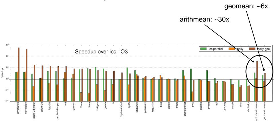
Xeon E5-2690 (10 cores, 0.5Tflop) vs. Titan Black Kepler GPU (2.9k cores, 1.7Tflop)
