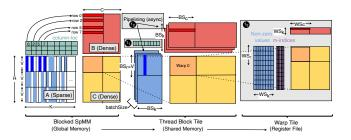
Figure 5: Thread-Block Tile and Warp tile view (stage 1)
