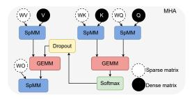
Figure 15: Simplified view of a pruned MHA
