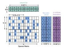
Figure 3: The V:N:M compression format
