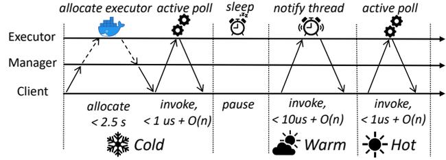
Figure 6: Lifetime of an *rFaaS* function. Similarly to serverless systems, the cold start times are dominated by sandbox initialization. Warm and hot invocation times include *rFaaS* overhead and latency of RDMA write of  $N$  bytes of payload.
