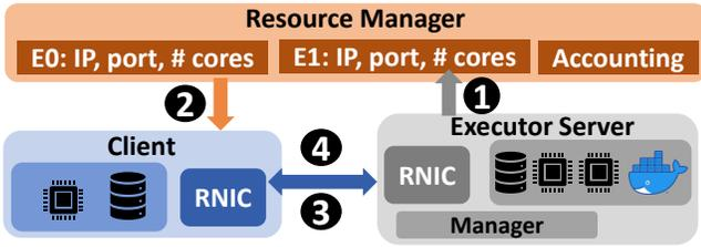
Figure 5: *rFaaS* system: resource manager receives (❶) and distributes (❷) computing resource availability, clients allocate executors (❸) and remotely invoke functions (❹).
