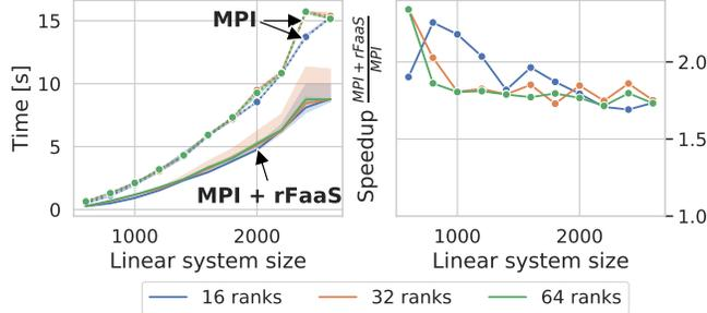
(b) Jacobi method, 100 iterations: MPI (dashed) and MPI+rFaaS (solid).
