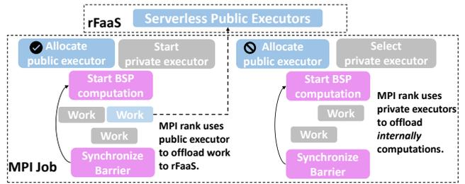
Figure 7: *rFaaS* for bulk synchronous programs: speedup without load imbalance even on limited resources.
