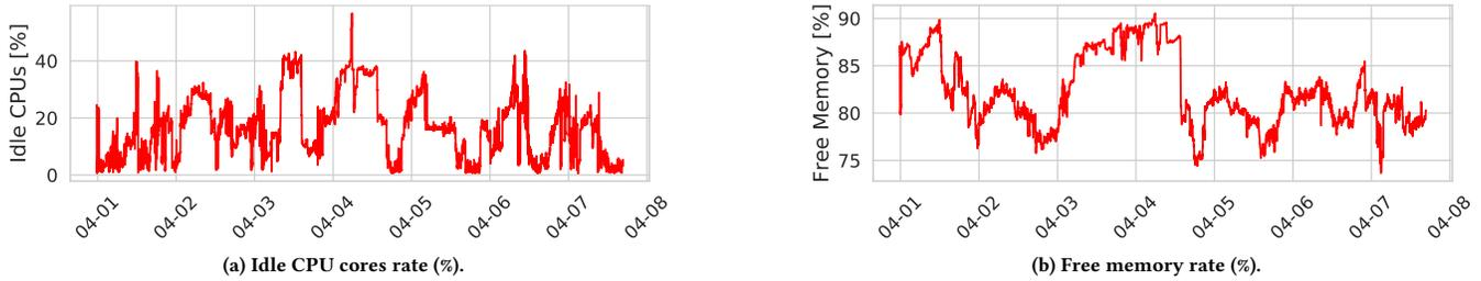
Figure 2: Piz Daint utilization for a period of one week (31.03-7.04 in 2021): querying SLURM with a one minute interval.
