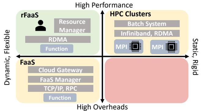
Figure 4: Comparison of execution systems for HPC: *rFaaS* offers the dynamic resource management of FaaS and performance comparable to batch systems from HPC clusters.
