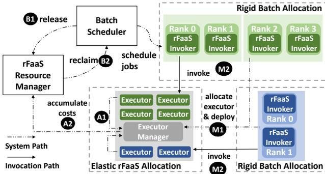
Figure 8: The system model of *HPC-as-a-Service*: *rFaaS* functions integrated with MPI applications (M), running on batch-managed clusters (B) with dedicated accounting (A).
