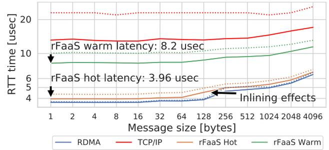
**Figure 10: The RTT of a no-op *rFaaS* function and network transport, median (solid) and 99th latency (dashed).**
