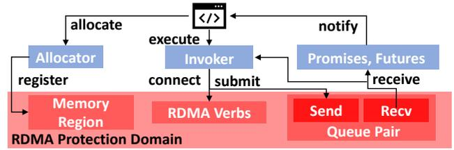
Figure 9: The *rFaaS* programming model. The model is inspired by C++ standardization efforts on the *executor* concept.
