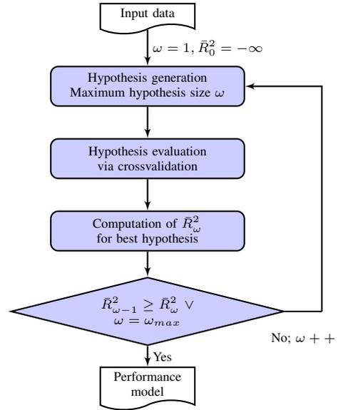
Fig. 1: Iterative model refinement process. Solid boxes represent actions or transformations, and banners their inputs and outputs [5].
